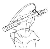
**5** Secure the two hexagonal bolts with the 3mm hexagonal wrench.
